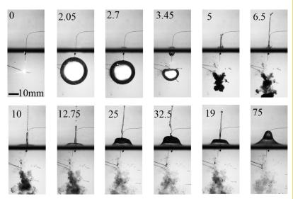
We have used a low-voltage spark circuit wherein a capacitor is first charged and then discharged through two contacting electrodes within a liquid to create a bubble. As the bubble expands and collapses, we observe dynamics of the bubble under different surroundings in both of the above mentioned problems. The entire dynamics were recorded using a high-speed camera which helped to understand the mechanism behind the observed behaviour.
