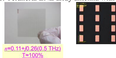
Fig. 7. Refractive index near zero and nearly perfect transmission by symmetrically aligned paired cut metal wires.
