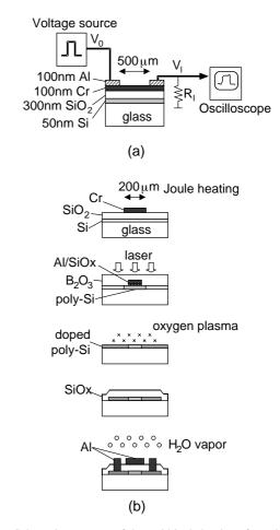
Fig. 1. Schematic apparatus of the rapid joule heating of metal films and the cross section of the layered structure of samples (a). 5- $\mu$ s-pulsed voltage was applied to 100-nm-thick Cr strip with a length of 500  $\mu$ m and a width of 200  $\mu$ m. (b) is schematic fabrication flow of poly-Si TFTs.
