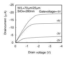
Fig. 4. Output characteristics of p-channel poly-Si TFTs with a channel length of 25  $\mu$ m and a channel width of 70  $\mu$ m.
