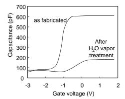
Fig. 3. C–V characteristics at 1 MHz for Al gate metal-oxide-semiconductor (MOS) capacitors with SiO<sub>x</sub> as fabricated and treated with  $1.3 \times 10^{6}$ -Pa-H<sub>2</sub>O vapor heating at 200°C for 3 h. The area of gate Al metal was  $5.5 \times 10^{-3}$  cm<sup>2</sup>.
