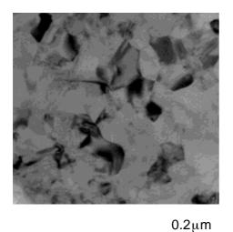
Fig. 2. Micrograph of the bright field image of transmission electron microscope (TEM) plane view for 50-nm-thick silicon films crystallized by the rapid joule heating of metal films at 140 V.
