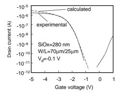
Fig. 5. Transfer characteristics of p-channel poly-Si TFTs. The solid curve is experimental drain current and the dashed curve is calculated drain current.
