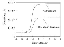
Fig. 2. Capacitance vs voltage characteristics with high frequency at 1 MHz for Al-gate MOS capacitors with 120-nm-thick  $SiO_x$  films for n-type substrates fabricated by thermal evaporation of SiO powders at room temperature in oxygen radicals. The area of the Al electrodes is  $0.01 \text{ cm}^2$ . High-pressure H<sub>2</sub>O vapor heat treatment was carried out at 260°C and 1.3 MPa for 3 h.
