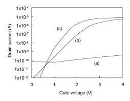
Fig. 3. Transfer characteristics for TFTs fabricated with no  $H_2O$  vapor heat treatment (a),  $H_2O$  vapor heat treatment after laser crystallization (b) and additional  $H_2O$  vapor heat treatment after TFT fabrication (c).
