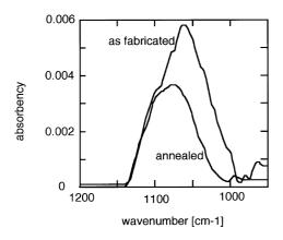
Fig. 3. Changes in the absorption spectra caused by the SiO antisymmetric stretching vibration mode by the heat treatment at  $270^{\circ}$ C with  $5.4 \times 10^{6}$  Pa H<sub>2</sub>O vapor for 3 h for SiO<sub>2</sub> layers formed using N<sub>2</sub>O plasma at 300°C for 1 h with a radio frequency power of 50 W and a gas pressure of 1 Torr.
