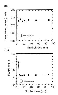
Fig. 2. Peak wavenumber of the absorption band caused by the SiO antisymmetric stretching vibration mode (a) and FWHM of the absorption band (b) as functions of the SiO<sub>2</sub> film thickness for the thermally grown SiO<sub>2</sub> samples. The SiO<sub>2</sub> layers were etched to different thicknesses after the heat treatment at 270°C with  $5.4 \times 10^6$  Pa H<sub>2</sub>O vapor for 3 h of 96-nm thick SiO<sub>2</sub> layers.
