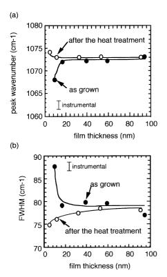
Fig. 1. Peak wavenumber of the absorption band caused by the SiO antisymmetric stretching vibration mode (a) and FWHM of the absorption band (b) as functions of the SiO<sub>2</sub> film thickness for the thermally grown SiO<sub>2</sub> samples with different thicknesses before and after the heat treatment at  $270^{\circ}$ C with  $5.4 \times 10^{6}$ Pa H<sub>2</sub>O vapor for 3 h.
