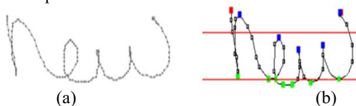
Figure 1: Preprocessing. (a) Original word (b) Preprocessed word – black dots denote feature points, red denote pen-down/up; blue and green denote maxima and minima respectively.
