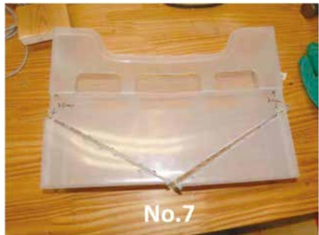
Fig. 5. Plastic document file case with a cutting line for buckets.
