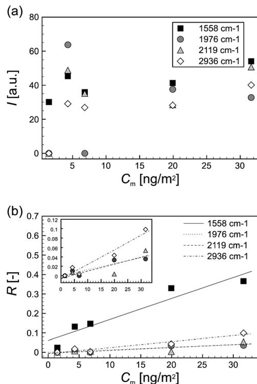
Fig. 7 Average Raman intensity,  $I$  (a) and occurrence frequency,  $R$  (b) with respect to peaks of 1558, 1976, 2119 and 2936 cm<sup>-1</sup> versus mass concentration per unit area,  $C_m$  (i.e.  $\sim U^{2/3}$ ); the regression lines are described for each peak.
