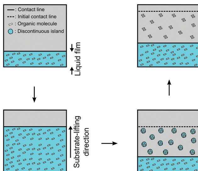
Fig. 4 A schematic illustration of development of discontinuous islands over a solid surface.
