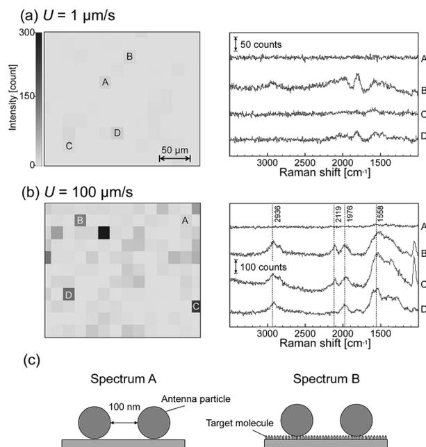
Fig. 6 Raman mappings (left) of peak intensities at  $1558 \text{ cm}^{-1}$  for the substrate-lifting rate ( $U$ ) of  $1$  (a) and  $100$  (b)  $\mu\text{m s}^{-1}$  and Raman spectra obtained from each measurement point (A to D, right). Formation of particle/substrate (spectrum A) and particle/molecules/substrate interfaces (c).
