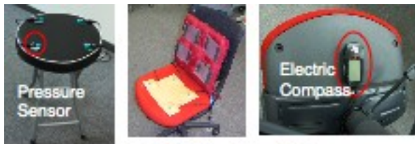
(a) Chair: Stool (left), office chair without (center) and with (right) an electric compass
