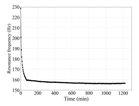
FIG. 2. Time dependence of the resonance frequency in Tube A. The depicted case used the gas mixture with a helium initial molar fraction of 50.0 %.
