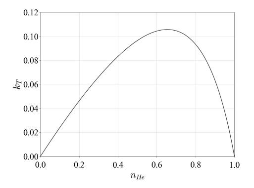
FIG. 9. Molar-fraction  $n_{He}$  dependence of the thermal diffusion ratio  $k_T$  from (Atkins *et al.*, 1939) results indicate that a multi-stage gas-mixture separation system can be used to obtain purer gas.
