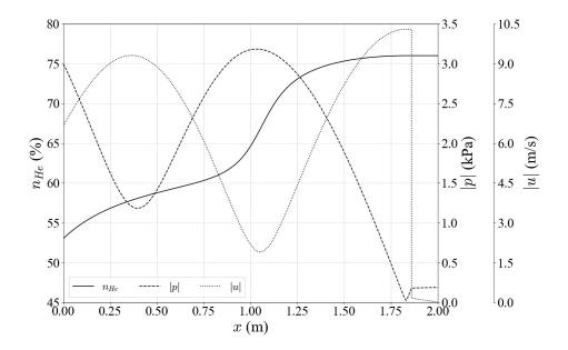
FIG. 4. Estimated acoustic and molar-fraction distributions in Tube B and C at the saturated condition. The commonly used thermoacoustic software DeltaEC was used for this calculation (Ward *et al.*).
