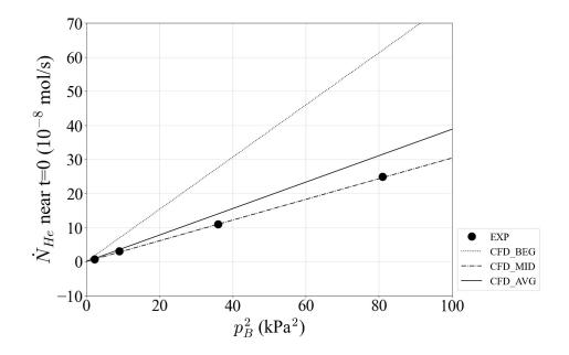
FIG. 5. Pressure-amplitude dependence of  $\dot{N}_{He}$  near t = 0. Note that the values are plotted as a function of  $p_B^2$ . Black-filled circles display the values estimated from the experimental results by Eq. (5) and (6). The calculated  $\dot{N}_{He}$  at the beginning (CFD\_BEG), midpoint (CFD\_MID), and the overall average (CFD\_AVG) of Tube B at t = 0 are plotted as a function of the pressure amplitude with lines.
