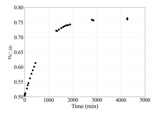
FIG. 3. Time dependence of the mole fraction  $n_{C,He}$ . The gas-separation experiment was conducted under the condition that the initial molar fraction  $n_{0,He}$  was 0.50, and the pressure amplitude  $p_A$ was 3.0 kPa.
