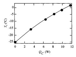
FIG. 8. Cooling power of the thermoacoustic Stirling cooler. Temperature  $T_C$  of the cold end of the second regenerator is plotted as a function of the load  $Q_C$ , when an input power  $Q_H$ =210 W. The line is a guide for the eye.
