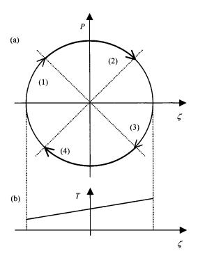
FIG. 1. (a) Relation between pressure P and displacement  $\zeta$  with the traveling wave phase. (b) Temperature gradient in a regenerator.
