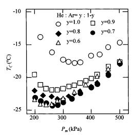
FIG. 7. Temperature  $T_C$  of the cold end of the second regenerator as a function of  $P_m$ , for input power  $Q_H$  = 210 W.
