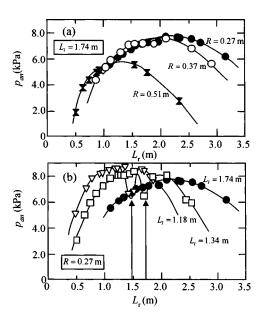
FIG. 3. The pressure amplitude  $p_{an}$  at the pressure antinode as a function of the resonator length  $L_r$  with (a) given distances R and (b) given looped tube lengths  $L_l$ . Curves are drawn to guide for the eye.
