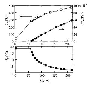
FIG. 6. Performance of the thermoacoustic Stirling cooler with the use of atmospheric air. Temperatures  $T_H$  at the hot end of the regenerator, in which the output power is generated, and  $T_C$  at the cold end of the second regenerator, in which the heat pump effect is operated, and square of pressure amplitude  $p_{an}^2$  are plotted as a function of input power  $Q_H$ . The lines are guides for the eye.
