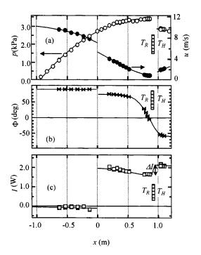
FIG. 4. Acoustic field in the thermoacoustic Stirling prime mover. The axial distribution of (a) p and u; (b)  $\Phi$ ; and (c) I. A hatched area represents the position of the regenerator and the lines are guides for the eye.
