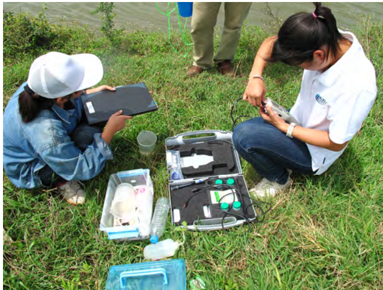
Photo 5a. Preparing the instrument before measuring the water qualities including EC, pH and temperature.
