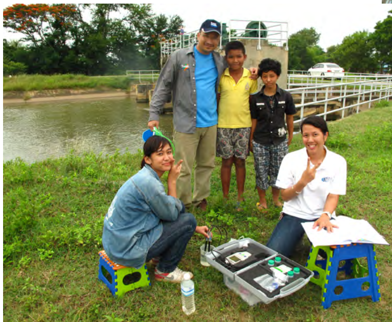
Photo 5a. Preparing the instrument before measuring the water qualities including EC, pH and temperature.
